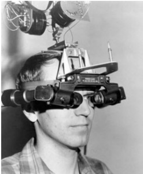
Figure 3 Sword of Damocles, the first VR headset
